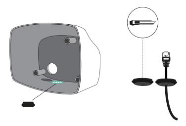
Make an incision in the rubber plug and insert the ethernet cable without the RJ45 connector. Ensure the cable is not too tight and has some clack to facilitate reopening the cover for possible maintenance or servicing. Crimp the RJ45 connector to the cable and connect the cable to the ethernet port in the charger.
